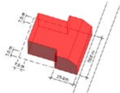
Current height, setbacks, and angular plane applied to a hypothetical 50m x 65m site.
